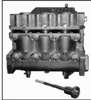
2) Lift discharge casing (50B) up and away.
